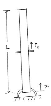
A 10 kg mass is attached to the top of a 10 cm long rod (E=20.×10<sup>10</sup> N/m<sup>2</sup>, and  $\rho=7800$  kg/m<sup>3</sup>). The other end of the rod is attached to a rigid foundation. The cross-sectional area of the rod is 1 cm<sup>2</sup>. What are the two lowest natural frequencies of the rod/mass for a longitudinal force applied to the mass in the direction along the length of the rod, as shown below?
