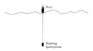
Fourier decomposition of the wave vertical motion yields vertical displacement of the hydrophone as a function of surface wave frequency. For example, at 100 Hz the vertical displacement magnitude is 100  $\mu$ m. Compute the apparent pressure signal (in Pa) picked up by the hydrophone due to this motion at 100 Hz. What is this pressure in dB referenced to 1  $\mu$ Pa?
