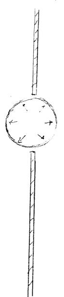
A flat 0.2 m diameter loudspeaker, with a diaphragm mass M of 15 grams and stiffness K of 3000 N/m is mounted at the end of an infinitely long rigid walled tube, as sketched in the figure below. Assume that the tube is filled with fluid with density  $\rho$  of  $1.41\,\mathrm{kg/m^3}$  and sound speed c of  $320\,\mathrm{m/s}$ , and that the diaphragm of the loudspeaker exactly matches the cross-sectional area of the tube.
